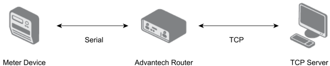
Figure 1: Serial2TCP router app function principle
